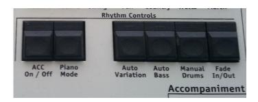
• ACC On / Off - This push button actives the Auto-Accompaniment for all Styles & Realdrums. The push button LED will light up RED when it is activated. When active, you will hear the full auto-accompaniment. If there is no sound, make sure that the grey accompaniment volume drawbars are not set to 0.
