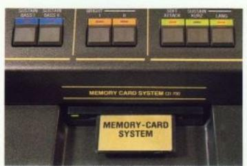
Software information is simply given to the SPECTRA by the Memory Card System. A storage system with no moving parts (unlike disk storage) and a physical size like that or a credit card.
