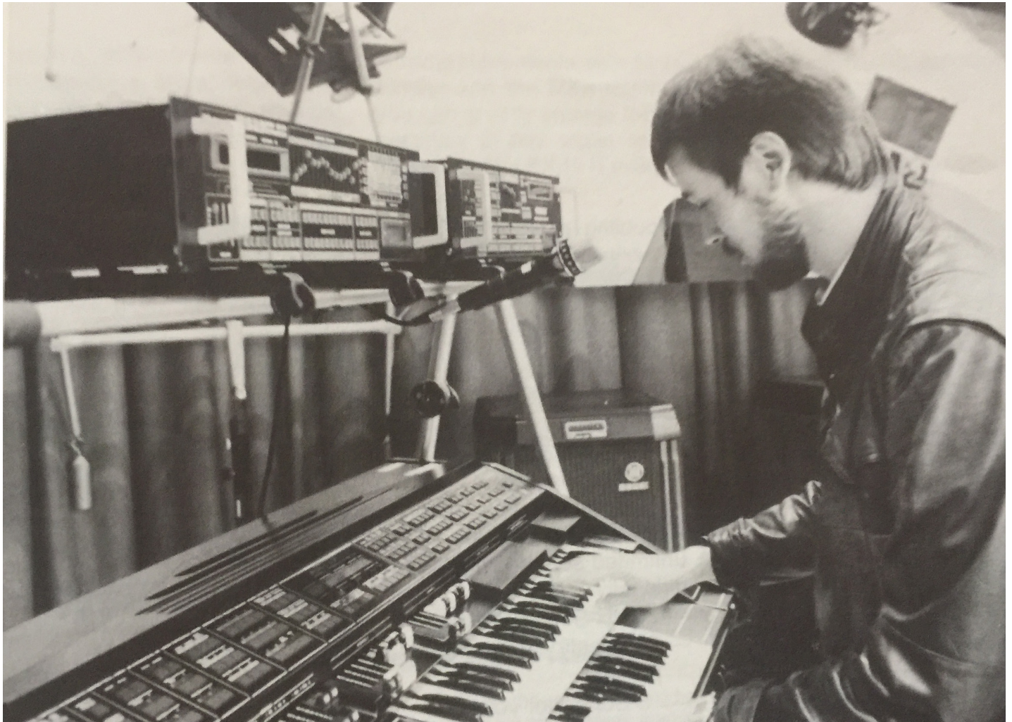
Above: MIDI set-ups shown at the Musikmesse featuring the EX20 and EX10 MIDI expanders linked to a WERSI Spectra via MIDI.
