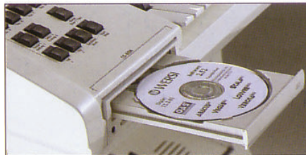
The integrated CD-Rom drive can also be used as a CD player.
